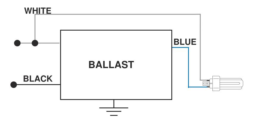
CAUTION: HIGH VOLTAGE: GROUND BALLAST CASE TO AVOID POSSIBLE SHOCK HAZARD. MOUNT LAMPS WITHIN 1/2 IN. OF GROUNDED METAL REFLECTOR.
