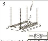
Connect the cable, L = black wire, N = whitewire, G= green wire. Please keep the circuit open during the process
