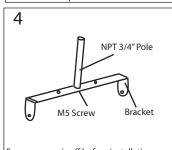
Ensure power is off before installation. Use M5 screw to lock the bracket and NPT pole.
