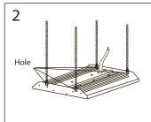
Lock the chain and hole on the housing. (Please keep the fixture horizontal)
