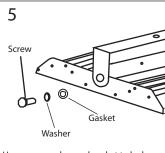
Use screw, washer and gasket to lock the bracket and fixture.
