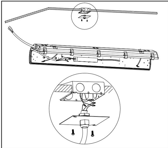
7. Reattach LED tray and lens to fixture by reversing step 4.
