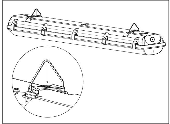
3. Hang fixture with the chains(not provided) using V-brackets.
