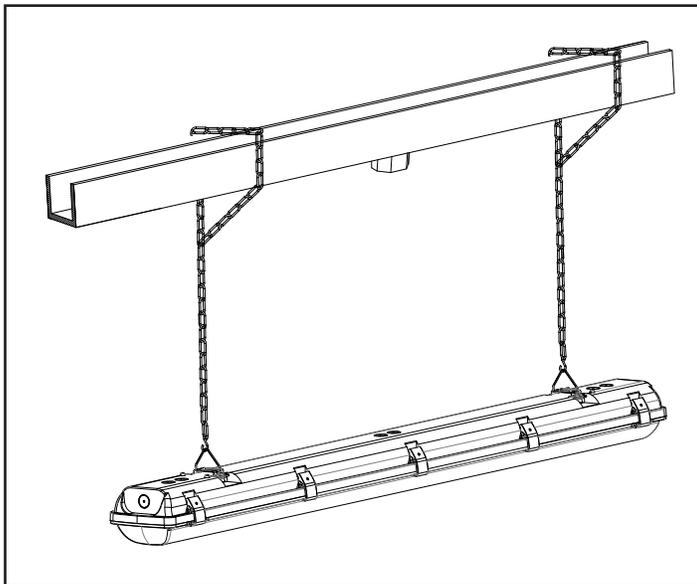
4. Release latches by pulling top of latch away from housing.
