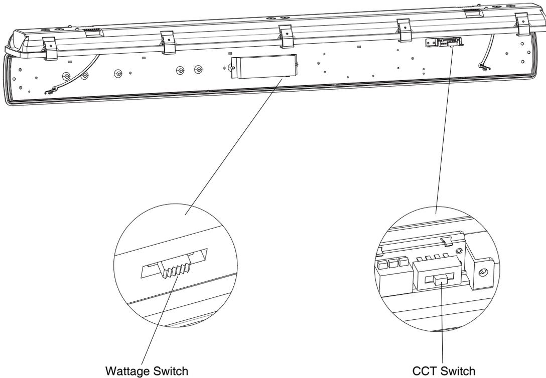
The end users may adjust the color temperature and lumen output respectively by the two DIP switch. Each DIP switch is accommodated with 3 options (left, middle and right), corresponding to 3 color temperatures and 3 powers respectively, which can perform the desired color temperature and lumen output combination.
