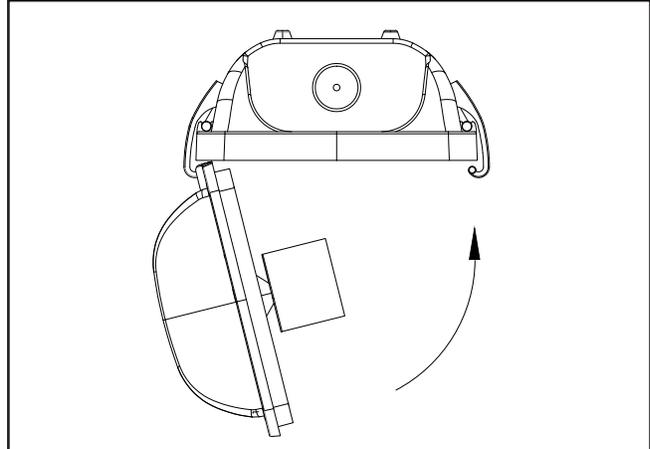
9. Secure lens to housing with lens latches.
