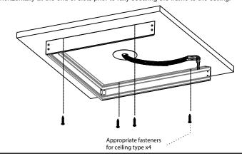
5.Put the wire conduit hose as close as possible to the surface mount opening before placing/inserting the luminaire into it partially. Make all electrical connections according to local code and make sure wire conduit hose is long enough for wiring connection in the surface of the surface
