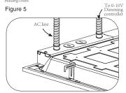
Plug in AC line(L and N, and GND) to the LED Driver using 18-14AWG Wire, When connecting 0-10Vdimming controller, wires must run through a separate knockout hole equipped with an appropriate electrical fitting. Figure 2
