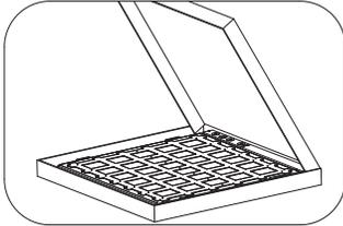
Carefully unpack unit and properly inspect for defects before installing. Wear work gloves to prevent dirt and oil from being transferred to the luminaire. If cleaning is needed, use gloves and a dry cottoncloth. It is not recommended to use hazardous chemicals.
