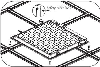
Insert luminaire into T-bar ceiling grid. Secure safety cable to meet local seismic requirements. Safety cable and method of attachment to the building provided by contractor according to local building codes.
