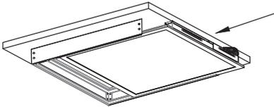
6. Push the conduit hose back into the surface mount frame properly, insert the luminaire fully into the frame. When installed properly, the luminaire will rest on the flanges of the surface mount frames. If the luminaire is not resting properly on the flanges, lift it up and shift it until it rests into place.
