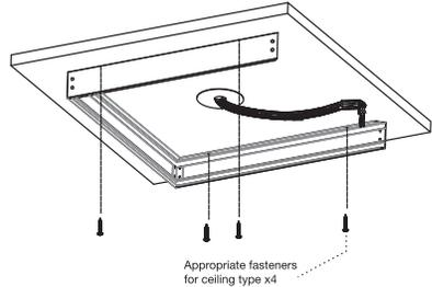
5. Put the wire conduit hose as close as possible to the surface mount opening before placing/inserting the luminaire into it partially. Make all electrical connections according to local code and make sure wire conduit hose is long enough for wiring connection job.
