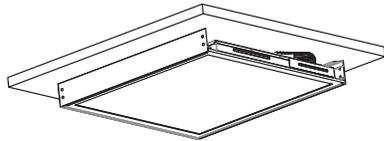
7. Place the last frame into the slots, then slightly slide the last frame to the left, make sure it get locked tightly, join the last frame to the rested frames by fastening them together with appropriate fasteners.
