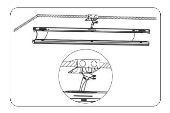
6.Assemble the module board upwards. The installation is completed.
