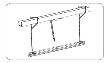
4.Connect the AC wires.
