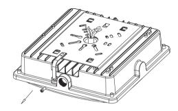
3. Screw the lamp and conduit pole together tightly.
