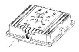
3. If you need to use the surface-mounted installation, a circle of sealent is needed around the edge of the fixed plate.
