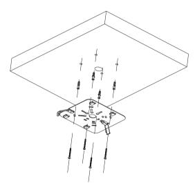
4. Buckle the connecting plate into the clips and connect the wires as shown below. PS: Wire the dimming wires (DIM+/DIM-) if needed, otherwise hide them in junction box.
