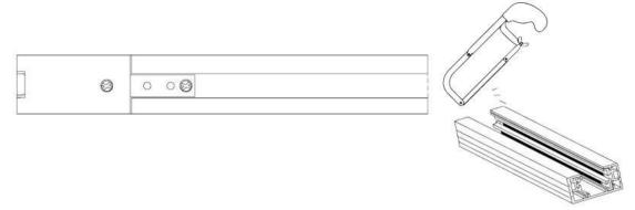
3. After achieving a flush cut, trim 1/4 inch off the end of each busbar. This will provide enough clearance for the end cap and ensure a proper connection with a mating connector. If this step is not followed in the correct order, the busbars may end up being too short, leading to faulty contact.
