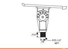
Wide-angle adjustable Kuckle Mount with angle indications of 30°,60°, or 90°. Heavy Duty Kuckle Mount supports the floodlight that best suits your needs.
